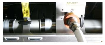
The handle (right above) next to the oil-disposal quickdisconnect activates the filter pump. All drain valves should be closed when oil is being pumped out for plisposal.
