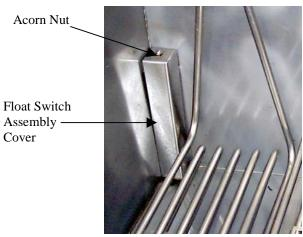
5. Clean crumbs and sediment around the float for proper operation. Reattach the float switch cover. It is important that this be done during every filtering process for proper operation of the fryer.
