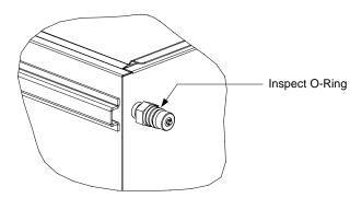
5. Push the prepared filter pan back into the fryer cabinet and reconnect the suction hose to the pan.
