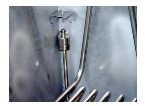
6. After cleaning the float switch and all oil has drained from the frypot into the filter pan, pull the filter pump T-handle to open the oil return valve and activate the filter pump.
